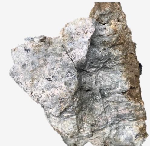
Epithermal Colloform Quartz and Ginguro Banding from the Maria Luz Sector
